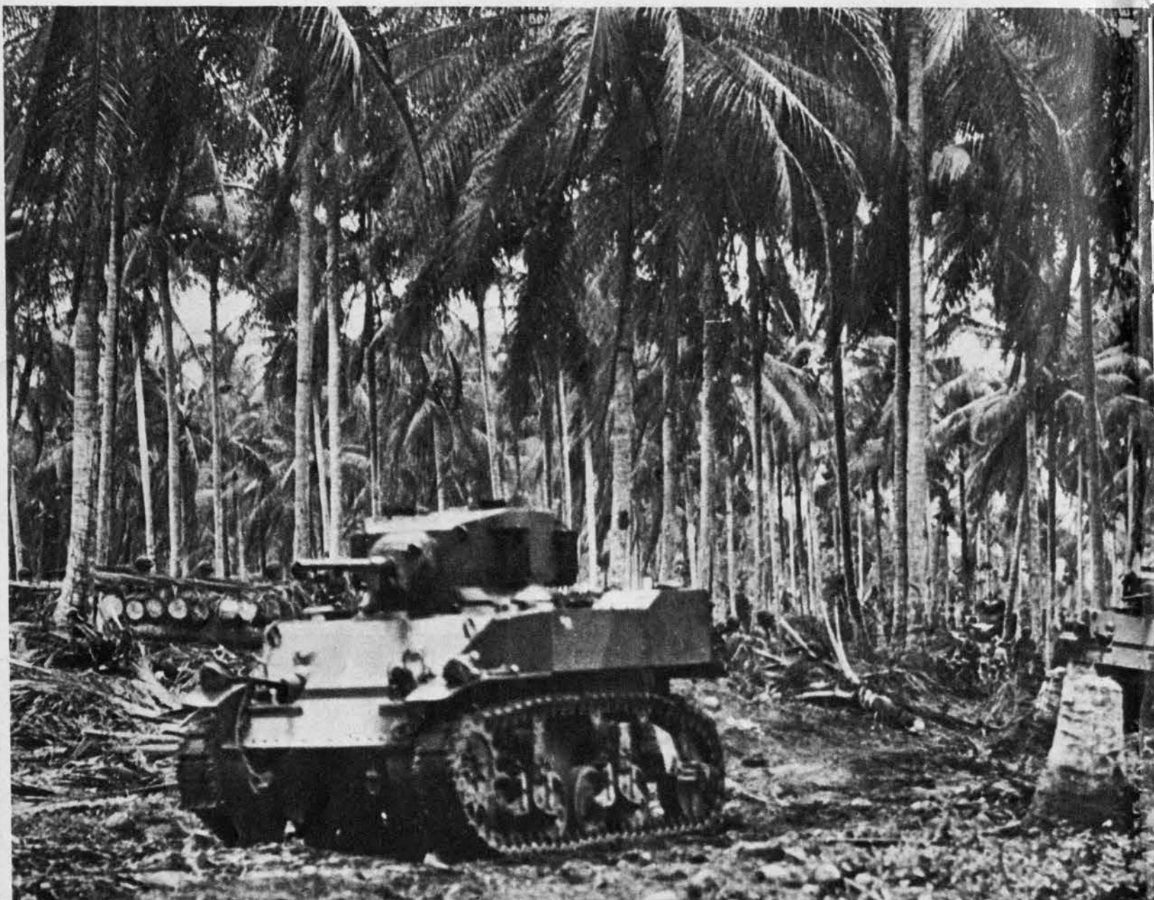
U. S. LIGHT TANKS LEAD THE WAY FOR INFANTRY AT ARAWE. M-5A1 HAS TWO PAIRS OF SMALL BOGIE WHEELS WITH PROMINENT BRACKET BETWEEN,
